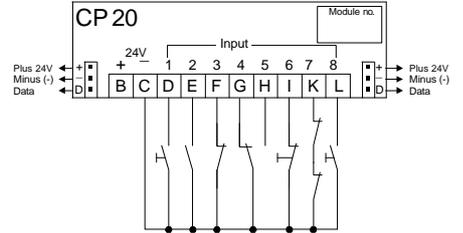
All inputs can be used individually, i.e. potential-free closing, opening or changing switches from touch button panels or other sensors can be used.
